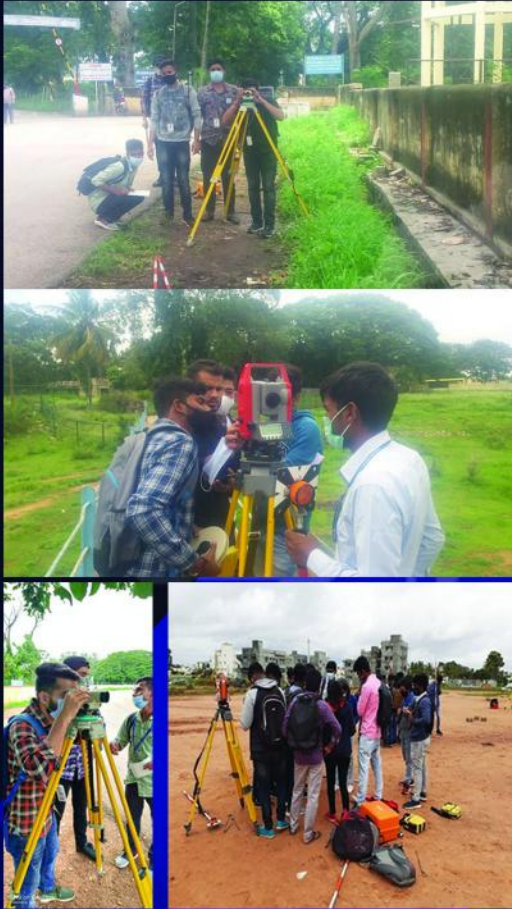
Students conducting survey using Dumpy level and Total Station equipments
